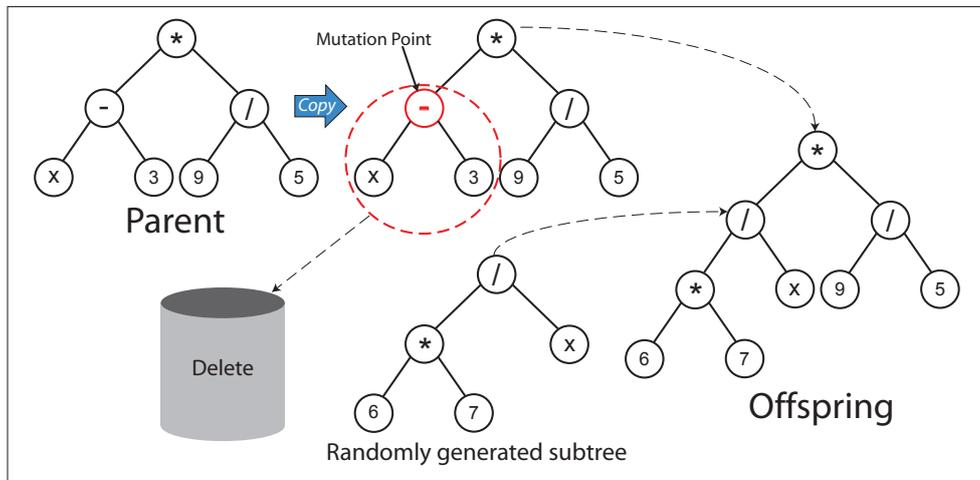
Figure 3.9: Illustration of GP subtree mutation.
