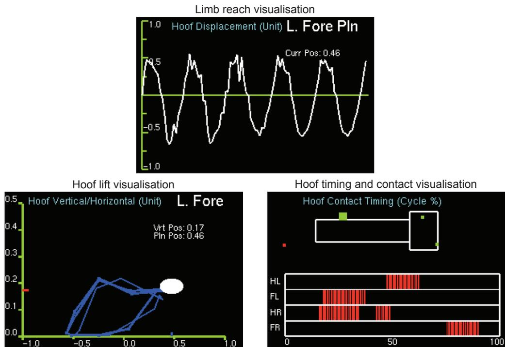
Figure 7.9: Three limb motion visualisations relating to limb and hoof motion.
