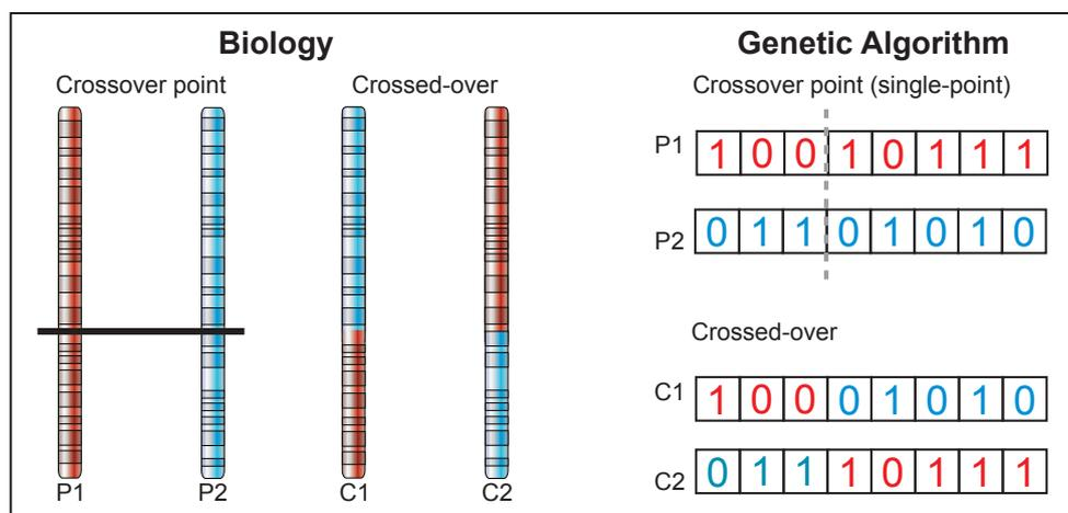
Figure 3.3: The images to the left depict crossover between two biological chromosomes (P=parent, C=child). The right of the diagram shows a single-point crossover between two GA chromosomes.
