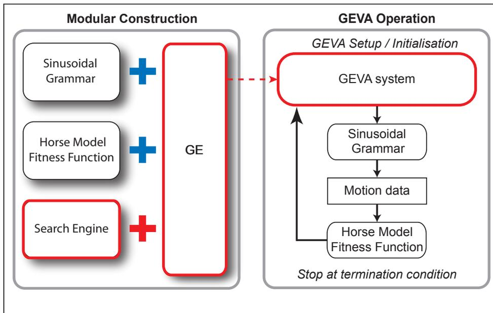
Figure 8.1: The modular construction of a GE system for motion data generation is shown in the image on the left. The implementation of such a system with GEVA is illustrated on the right.
