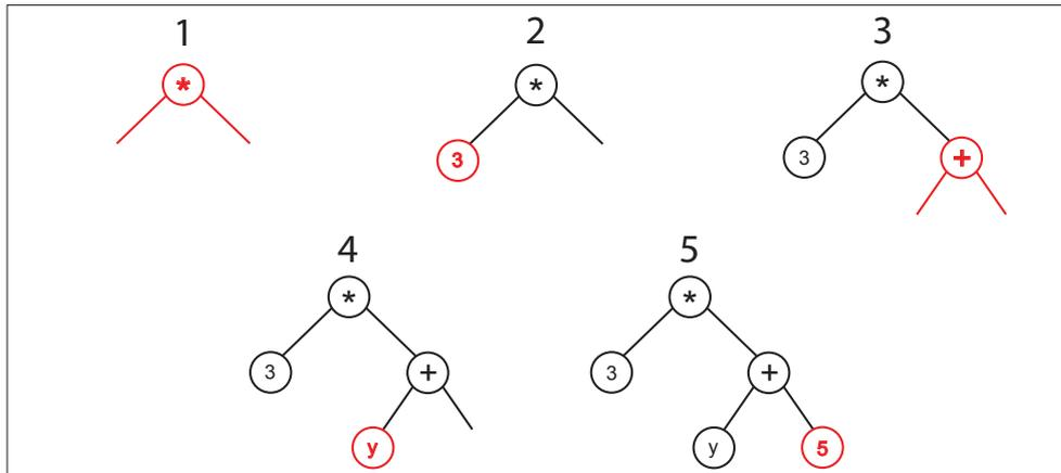
Figure 3.7: Grow initialisation: steps taken in creating a tree with a maximum depth of 2.
