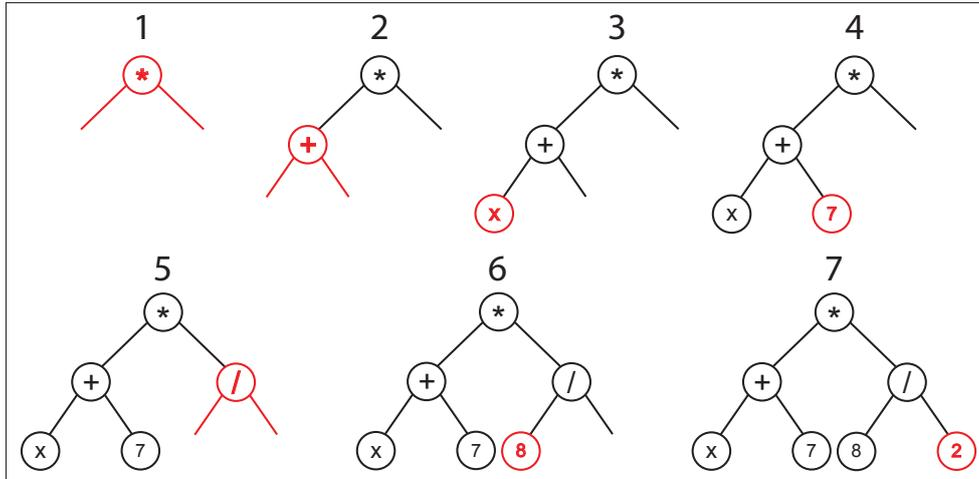
Figure 3.6: Full initialisation: steps taken in creating a tree with a maximum depth of 2.
