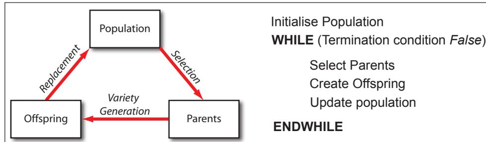
Figure 3.1: The cycle of natural evolution and the basic evolutionary algorithm pseudocode.
