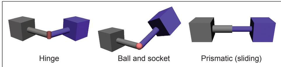
Figure 2.5: Three commonly used joints in computer animation.
