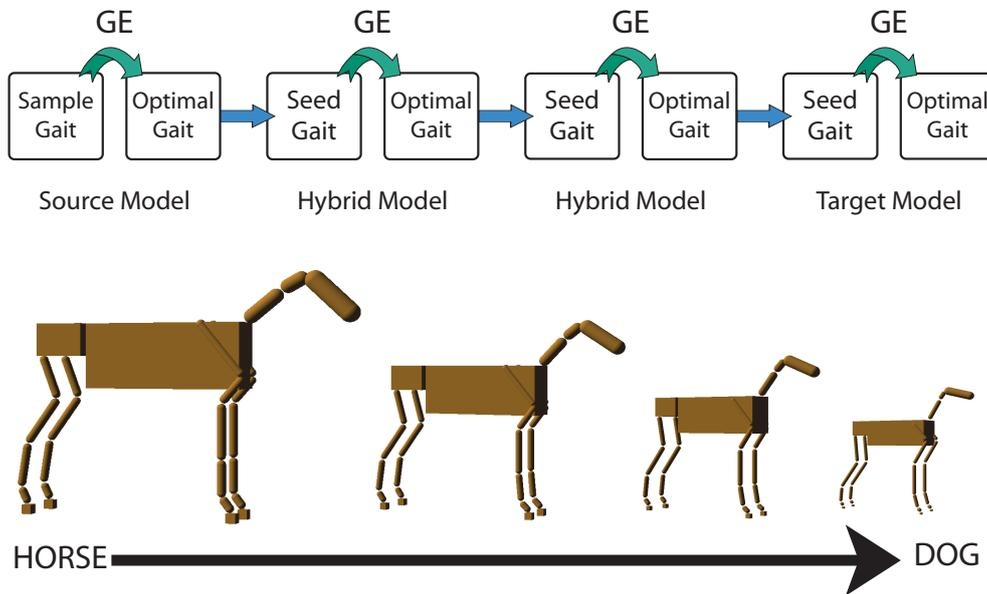
Figure 9.1: Discrete motion data retargeting with Grammatical Evolution (GE). Optimisations are performed on a series of intermediate horse-dog hybrid models.
