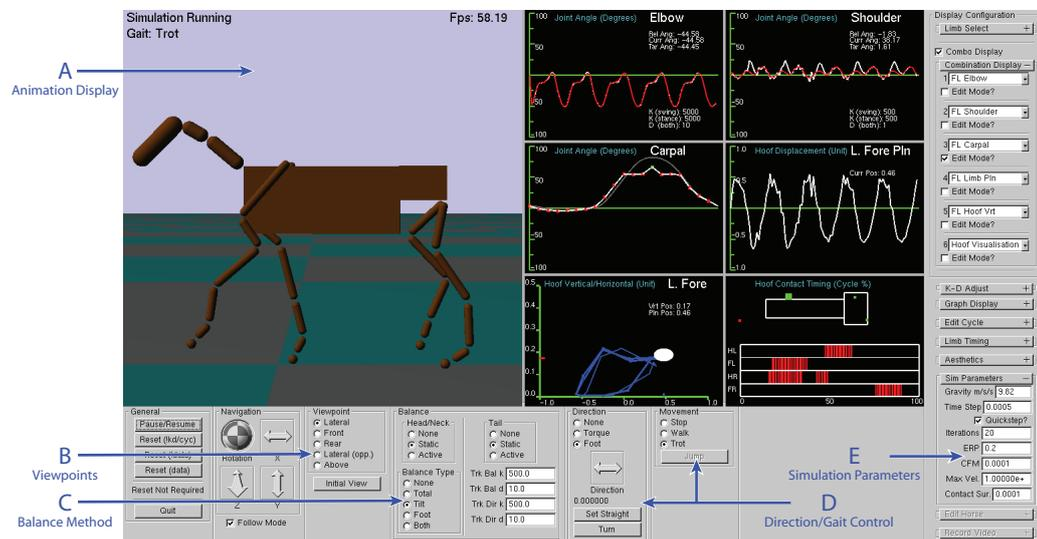
Figure 7.6: Annotated screenshot of the Motion Data Development Environment (MDDE).
