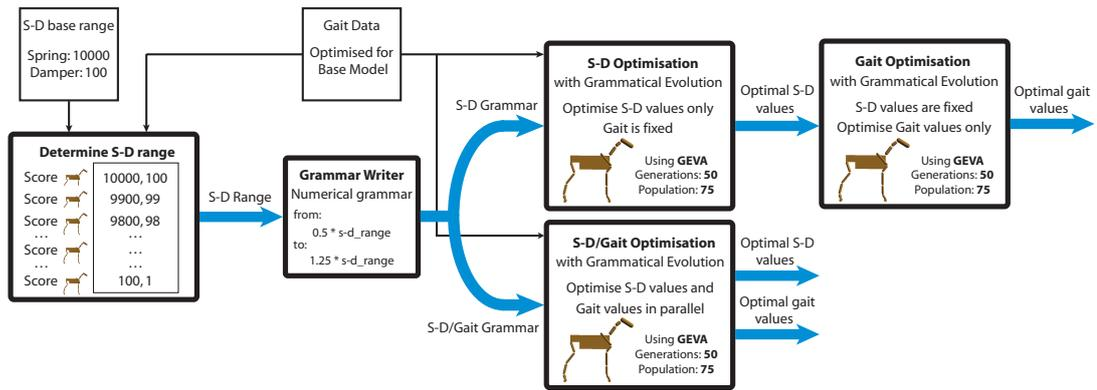
Figure 9.5: Flow chart of the spring-damper (s-d) coefficient and gait optimisation process. Note: the two distinct approaches investigated are distinguished by the fork in the flow chart.
