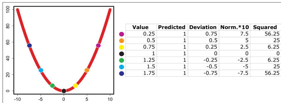
Figure 8.2: The fitness curve used to score each fitness component is shown alongside an example of how fitness scores are calculated. Fitness weights are not included in this example.
