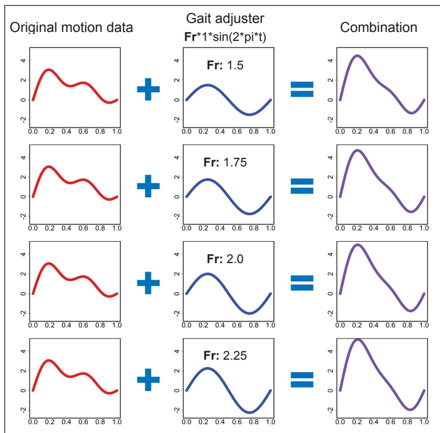
Figure 10.1: Illustration of the gait adjuster system. Each adjuster is a function of the current Froude number  $Fr$  and is added to the current gait's motion data to produce the motion with which the model is animated.
