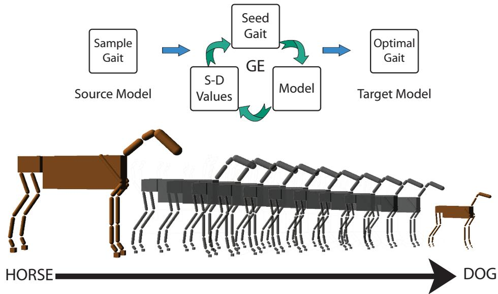
Figure 9.2: Continuous motion data retargeting with Grammatical Evolution (GE). Optimisations are continuously performed on the seed data, model's proportions and s-d coefficients until the target is reached.
