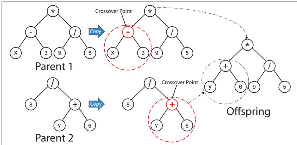
Figure 3.8: Illustration of GP subtree crossover.
