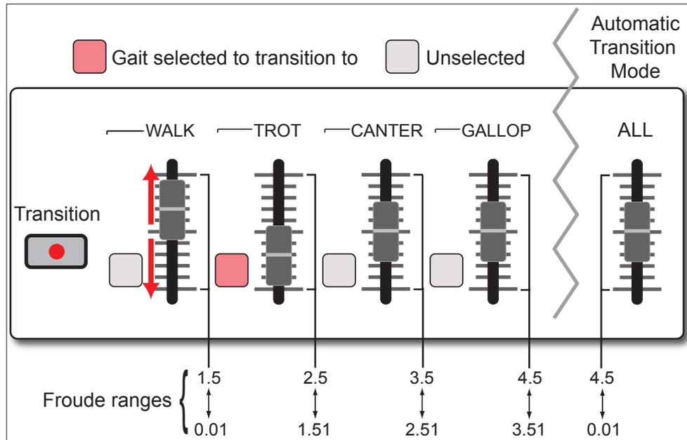
Figure 10.4: Simplified illustration of the MIDI controller. A user selects a gait for transition, sets the slider to a Froude value and then presses the Transition button.
